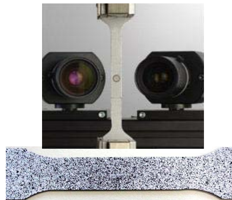
(b) ARAMIS ® setup and surface treatment
