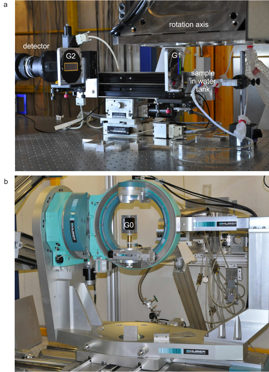
Figure 3.5.: The grating interferometer setup at the beamline W2. (a) The part downstream of the sample, which is mounted hanging down from the rotation stage into a water bath, consists of the phase grating G_1 , the analysing absorbing grating G_2 , and the detector including the lens system and the blackened luminescence screen. (b) The source gold grating G_0 is mounted 3.0 m upstream of the grating G_1 .
