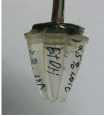
Figure 4.1.: Picture of the fluid phantom constructed for the measurements at the synchrotron radiation source. The bottom region of the phantom was scanned, where the outer diameters of the tubes are \approx 5 mm.
