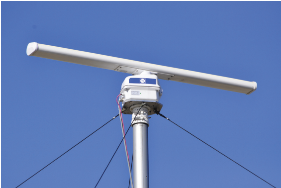
X-Band radar antenna
